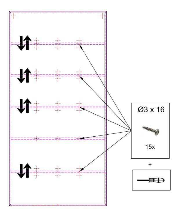
For loads over 5 kg, we recommend connecting the shelf with the rear wall.
